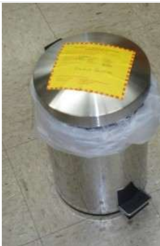
Ethidium bromide waste is to be collected in a leak-proof container with a lid lined with a sturdy, non-descript bag. The UT Hazardous Waste label should be placed on the storage container as well. No biohazard labels!
