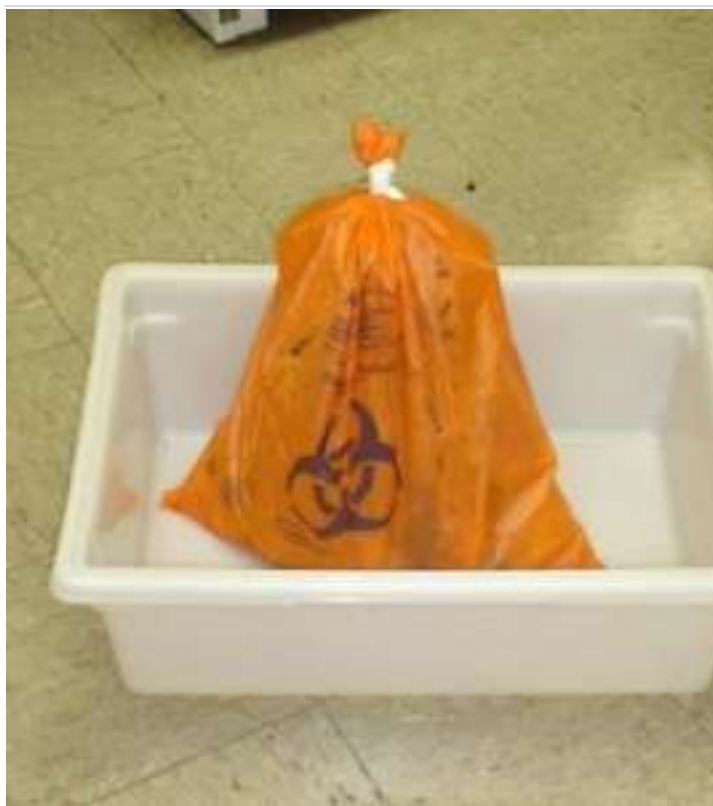
Biohazardous waste bags awaiting treatment should always be stored in pans or secondary containment to prevent spills!
